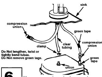
Use a compression union to connect the longer, 1/4" tubing from the faucet to the back tubing in the top of the
